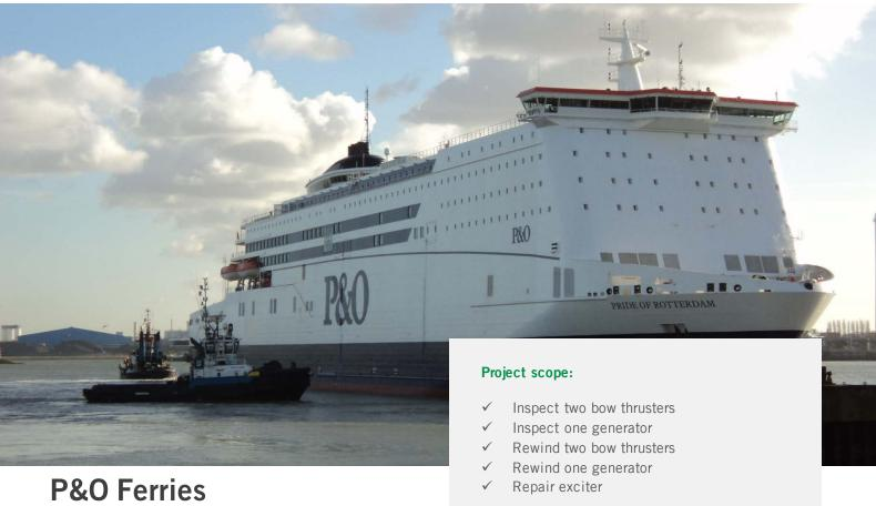
Multiple repairs on bow thrusters and generators – 2015
