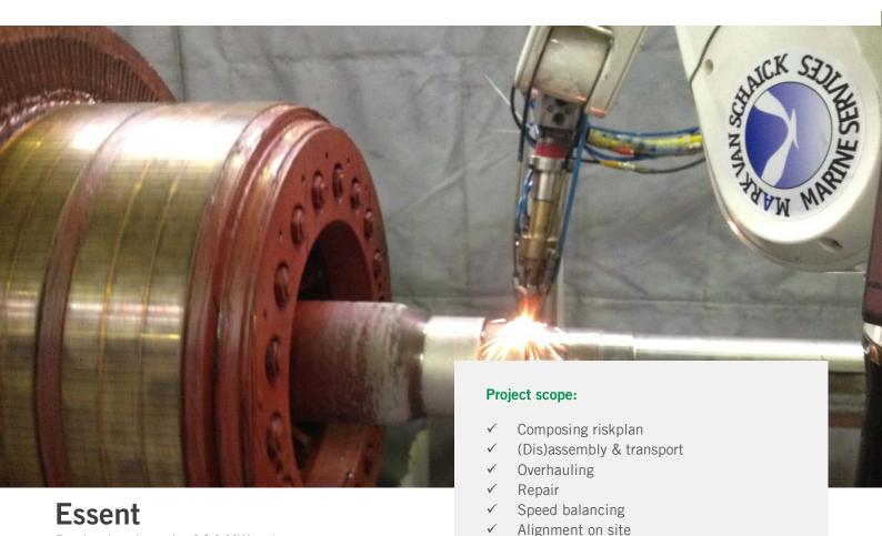
Essent, an energy company that provides gas, electricity and heat to consumers and businesses, ordered Bakker Repair + Services to replace the bearings of a 14 MW water pump onsite. Bakker Repair + Services discovered severe damage to multiple slide bearings and advised Essent to perform additional repairs.
